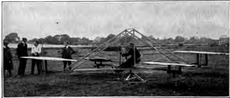
Fig. 37. Monoplane Dummy Used for Practice in Aviation Schools
